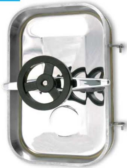
Rectangular manhole door in AISI 304 or AISI 316 stainless steel - frame in flat stainless steel or iron - vertical inward opening - access 500 x 310 mm.
