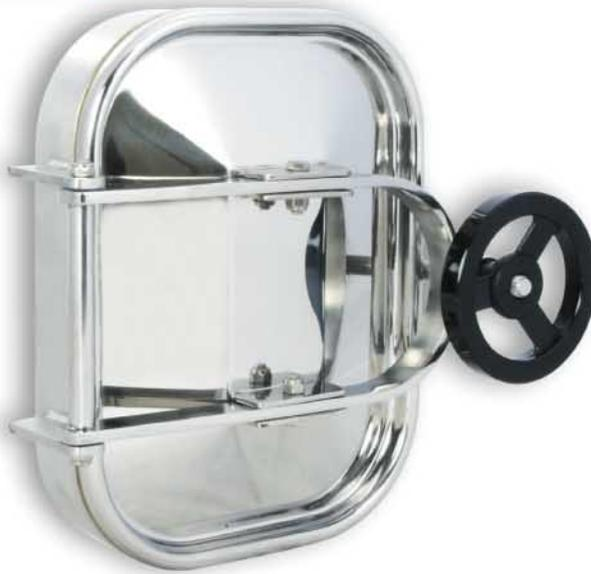
Rectangular manhole door in AISI 304 or AISI 316 stainless steel - frame in flat stainless steel or iron - outward opening - access 420 x 310 mm.
