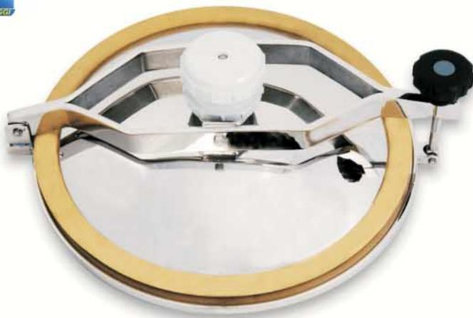
Upper lid "export" type in AISI 304 or AISI 316 - with 50 dia - pressure compensating valve - vertical and horizontal opening - access 420 mm.
