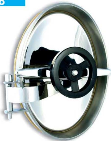
Oval shaped manhole door in AISI 304 or AISI 316 stainless steel - vertical inward opening with support arm - frame fabricated in flat stainless steel or iron - access 440 x 310 mm.
