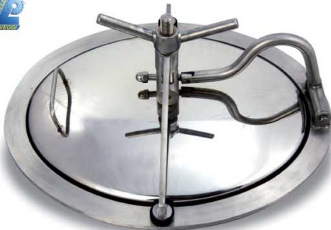
Oval shaped manhole door in AISI 304 or AISI 316/L stainless steel - inward opening - frame fabricated in flat stainless steel 40x10 access 520 x 420 mm.
