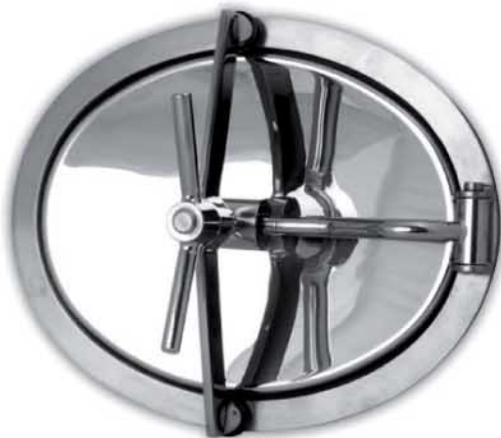
Oval shaped manhole door in AISI 304 or AISI 316/L stainless steel - inward opening - frame fabricated in flat stainless steel 30x12 access 440 x 340 mm. Certification PED.
