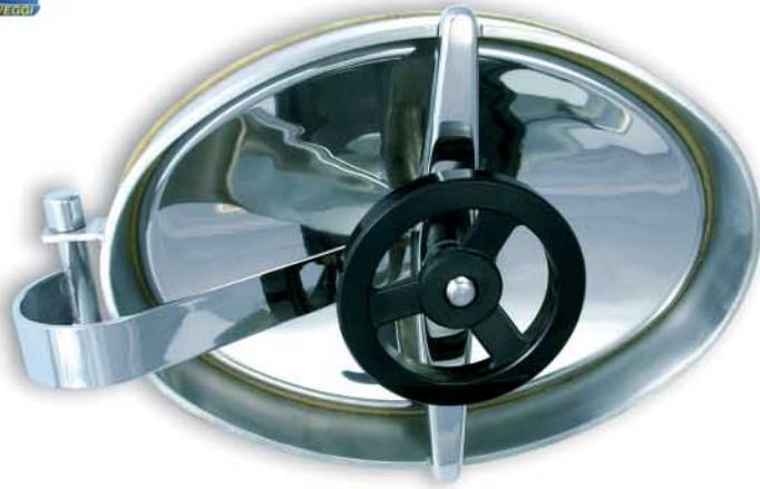
Oval shaped manhole in AISI 304 or AISI 316 stainless steel - horizontal inward opening with support arm - frame fabricated in flat stainless or iron - access 440 x 310 mm.
