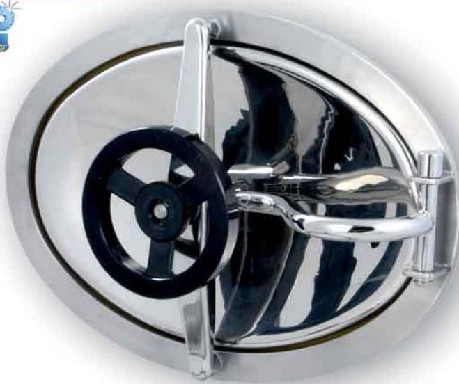
Oval shaped manhole door type "fruit juice" in AISI 304 or AISI 316 stainless steel - inward opening - frame fabricated in flat stainless steel - access 440 x 310 mm. (available on request with bending for various vat diameters).
