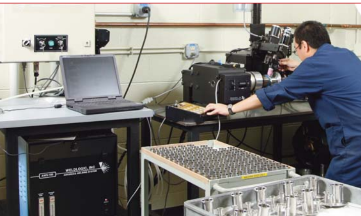
Where high precision welds are required, a welding lathe with a laser seam tracker is used to weld the parts.
