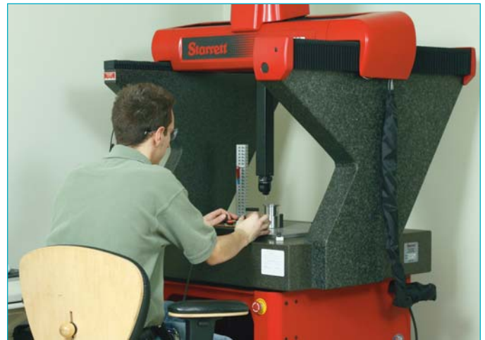
Eagle uses a Coordinate Measuring Machine (CMM) to check the dimension and tolerance of the parts.
