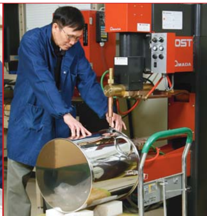
A spot welder is used to spot weld some parts onto the larger vessels.
