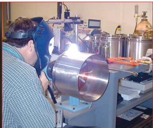
This Automatic Rotating Positioner is used to weld a flange to the vessel.
