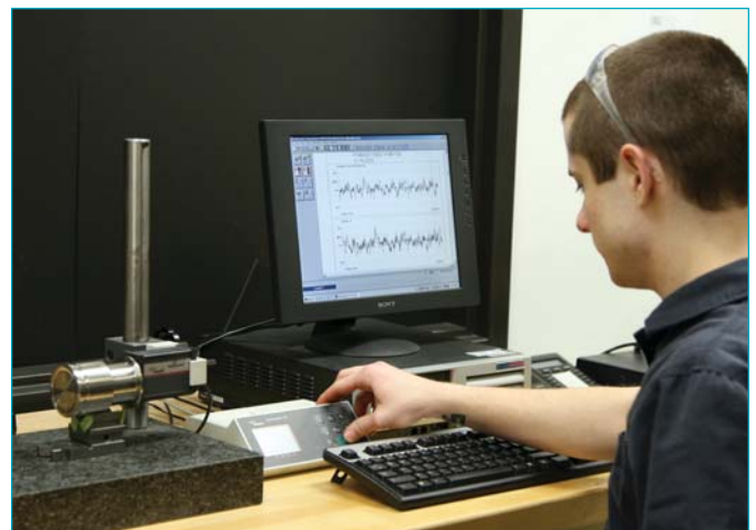
Roughness Average (Ra) is measured using a surface testing instrument.
