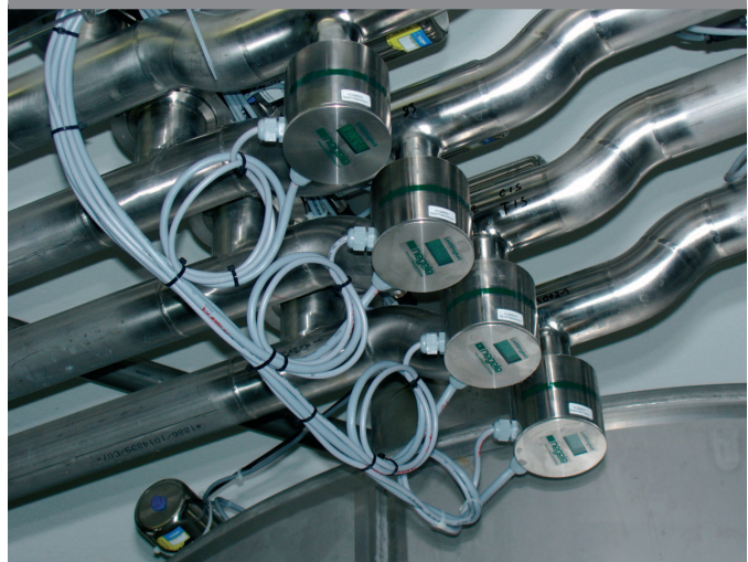
Phase separation in CIP-equipment with ILM-2
